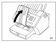
Lift up on the Document Exit Tray so that it catches under the Control Panel.
